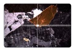
4. Loosen the stage brake and rotate the stage until the noticeable point of the sample is furthest away from the center of the crosslines. This may even be outside of the field of view. This indicates the objective is not centered to the stage.
